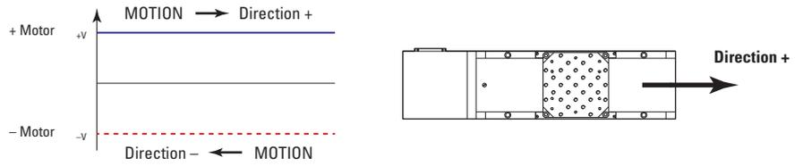
In the above drawings, + Motor signal is referred to - Motor signal.
