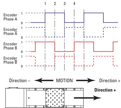
The incremental sensor consists of an optical scale and an encoder head. When the carriage moves, the encoder head generates square signals in quadrature and sends to pins #19, #20, #23 and #24 of the SUB-D25 connector.
