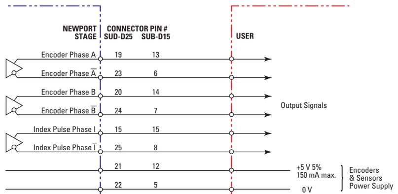
“Encoder” and “Index Pulse” are “differential pair” (type RS-422) type output signals. Using these signals permits a high immunity to noise. Emission circuits generally used by Newport are 26LS31 or MC3487. Reception circuits to use are 26LS32 or MC3486.
