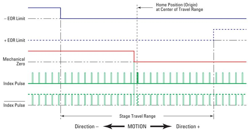
End-of-Run and Mechanical Zero are 5 V open collector type.
